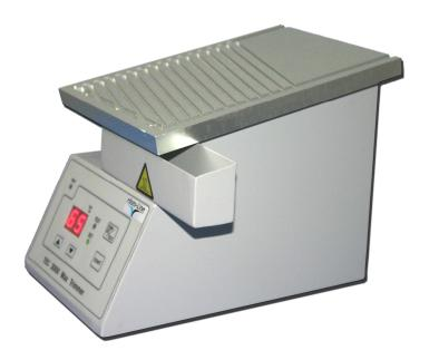
TEC 3000 Wax Trimmer is a safe and practical instrument designed for removing excess paraffin from tissue cassettes following embedding. Simply slide paraffin blocks across the heated grooved plane surface, excess of paraffin
