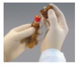
Sealed Aeroshields hold tubes up to 10 mL (16 x 100 mm) and—with their threaded, screw cap design and o-ring closure—provide full aerosol containment. The transparent cap allows you to inspect tubes for breakage without opening the seal. Aeroshields may be autoclaved and decontaminated with bleach.
