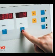
Set the required speed and the required time. With the "start" button, repeat runs can easily be recalled.
