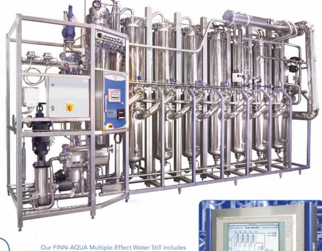
Our FINN-AQUA Multiple-Effect Water Still includes a user-friendly touchscreen and is available to order with either the latest Siemens or Allen-Bradley control system platform. Process display also available.
